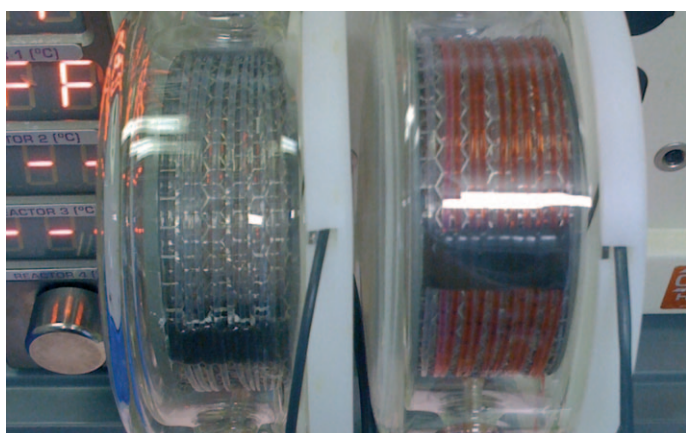
Figure 2. Bright red colour observed during the amide coupling reaction at 25 °C.
